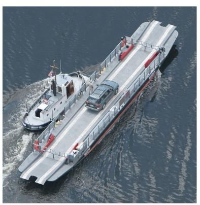
*Hollister III*. The three-car barge is towed back and forth by the *Cumberland*, a diesel powered towboat.
